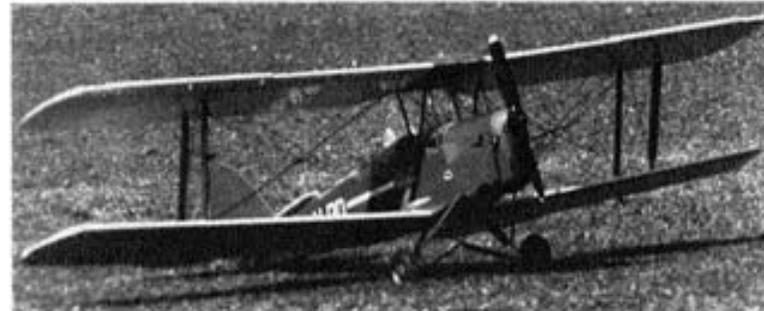
No, the picture is not back to front. The prop is left-handed! Harold's Merco 49 has been modified to clockwise rotation for true scale effect. Check that the side thrust on your model is suited to the crankshaft direction of the motor to be used.
