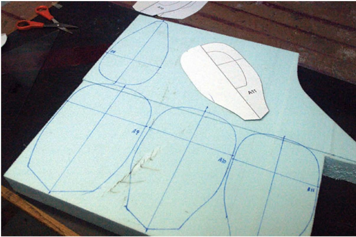
The fuselage section patterns are cut from the plans and used to mark a 1.5-inch thick sheet. Extruded sheet foam is available at most home improvement stores. Using a scroll saw is the best method to cut it.
