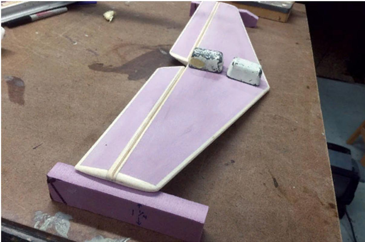
The horizontal stabilizer is shaped using sanding guards at the root and tip because the surface is so thin. The hinge line and edges have balsa bonded to them for protection and additional strength before the 1/2-ounce fiberglass cloth is applied.
