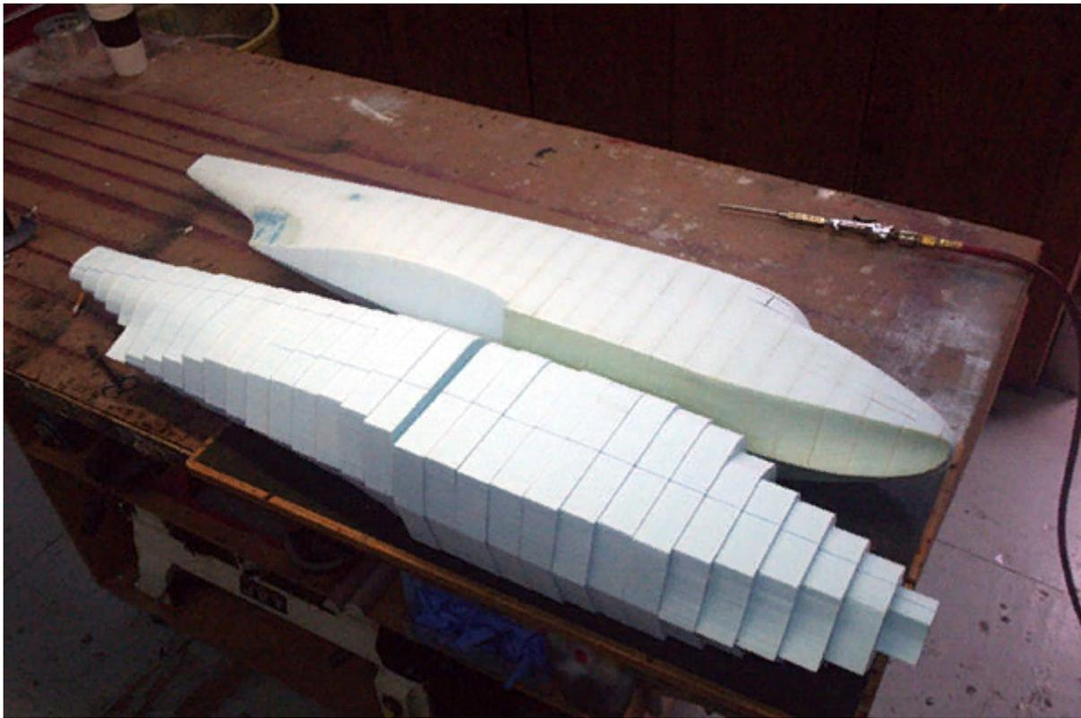
**Before and after:** This method greatly reduces the time required to shape the fuselage and increases accuracy. Because you only sand off the corners of the sections, it is surprisingly quick.
