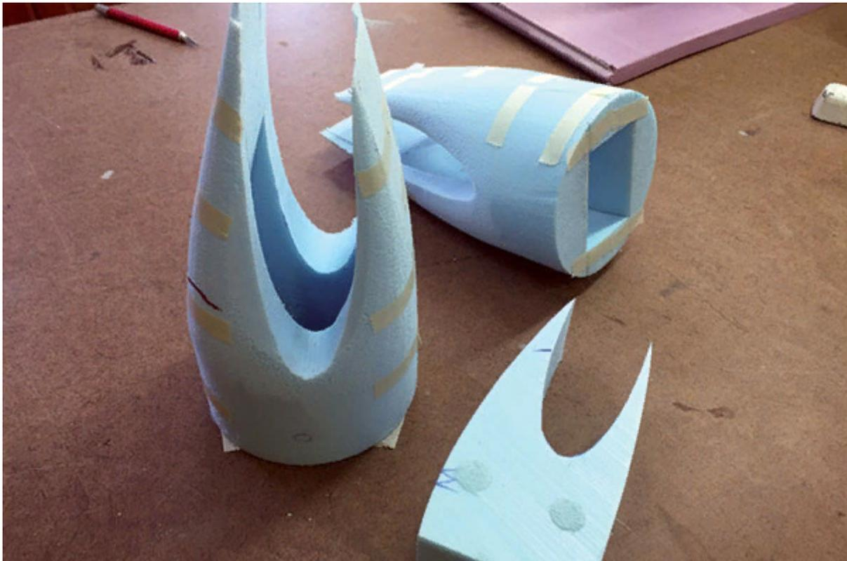
**The nacelles are made from three pieces of sheet foam using the patterns from the plans. They are tack-bonded together, sanded to the round shape, then disassembled to remove the center portion to house the ESC.**
