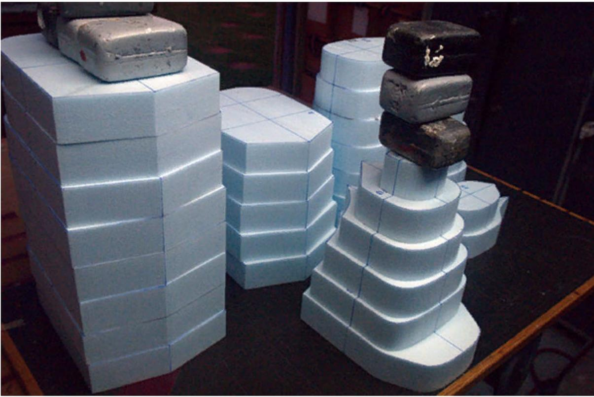
**The sections are tack-bonded together to prepare the fuselage for shape sanding. It is best to only manage a few bonds at one time to be sure the centerlines and waterlines stay aligned.**
