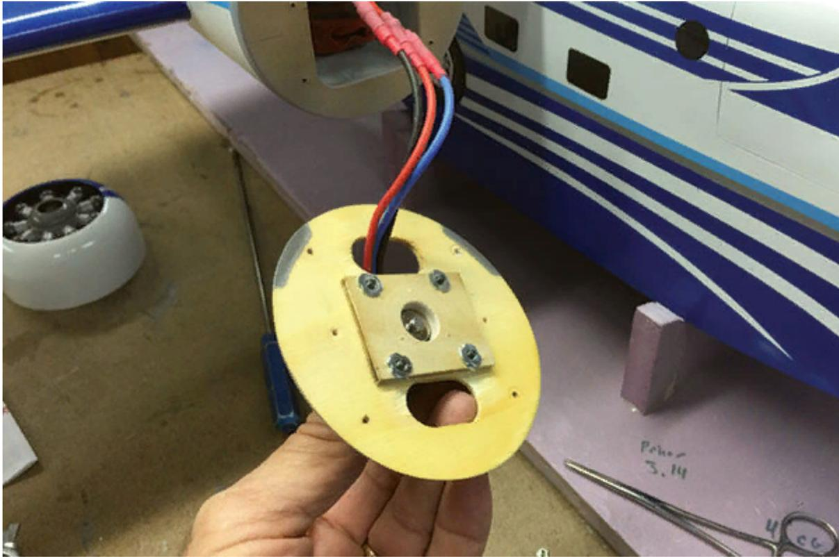
The firewall is made up of three light plywood parts that provide motor and cowl support as well as access for ESC servicing. Assembly is done with internal hex-head wood screws through the cowl.
