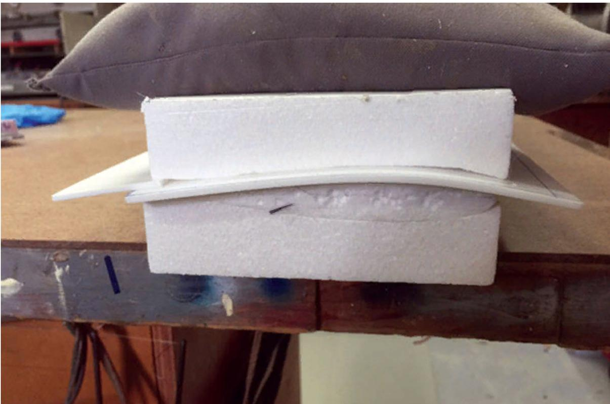
**Gorilla Glue is used to bond the foam sheeting to the foam core. Sandbags and the foam bed are used to apply pressure evenly for a complete bond. The drying time is overnight.**
