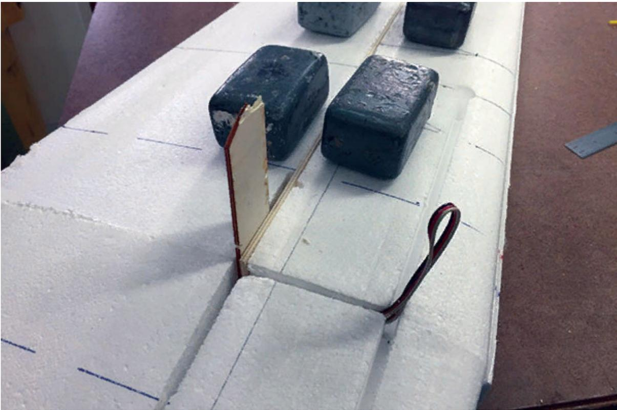
**After the wing cores are joined and the top sheeting has been installed, channels are cut in the foam to install the wiring and the main spar.**
