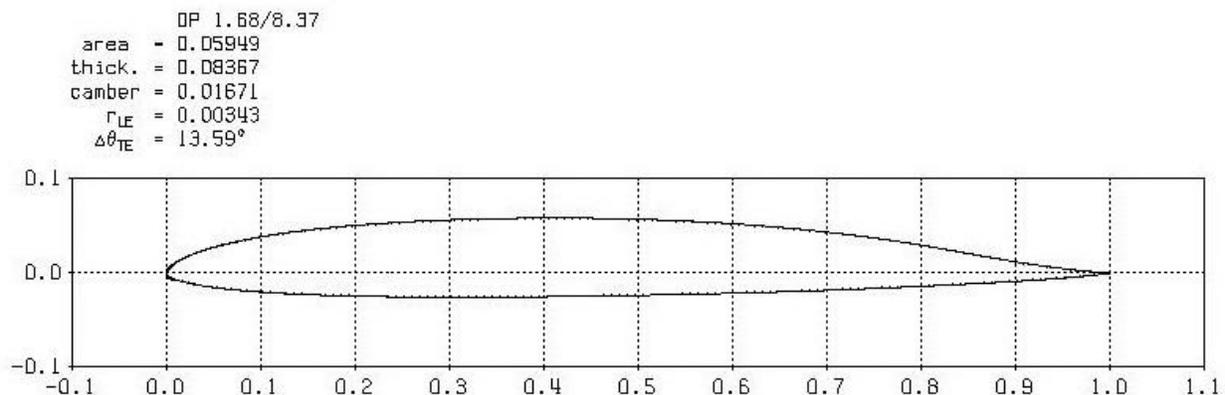
That airfoil has maximal thickness of  $8.37\%c$  at the distance of  $x=38.7\%c$ , and the maximal camber of  $1.67\%c$  at the distance of  $x=46.3\%c$ .
