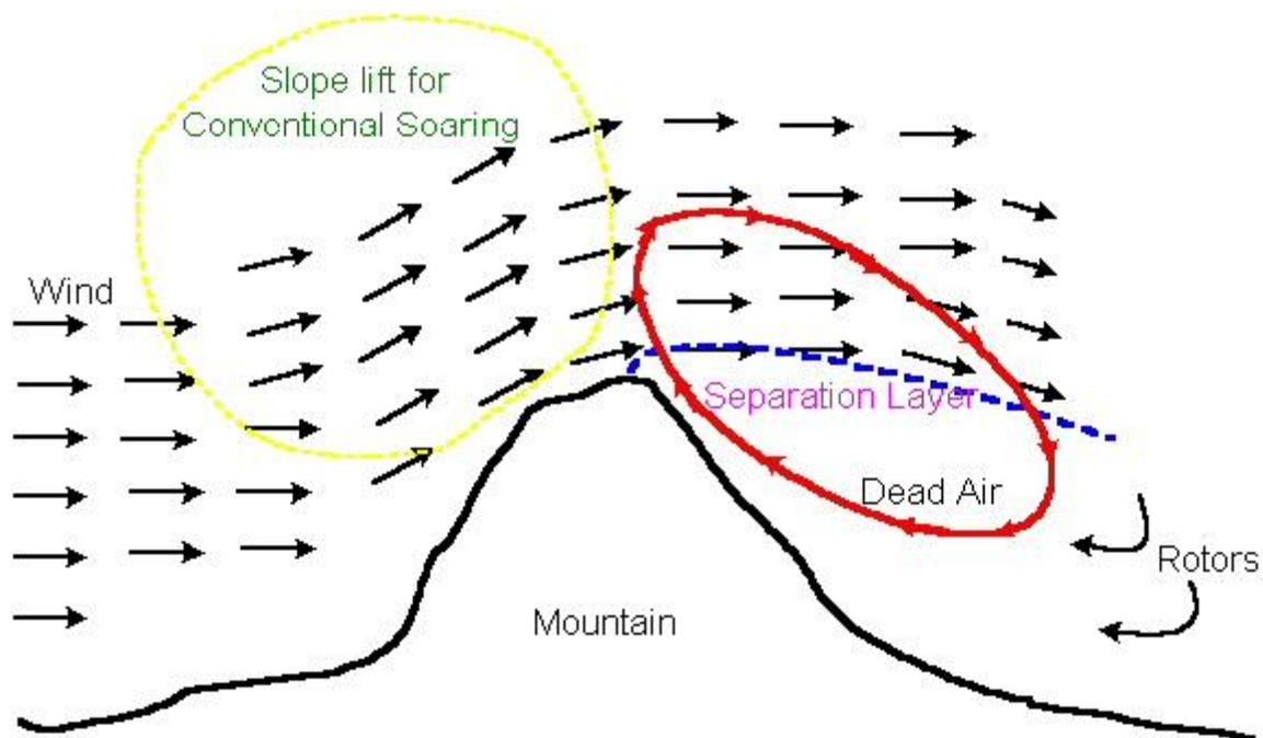
On the left side of picture long glider soaring on slope use lifting component of wind but on the right side of picture glider fly in circles get energy from wind only on the top of cycle (above separation layer) but longer path is in the dead air behind mountain.
