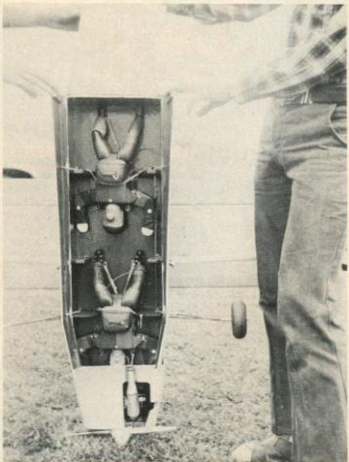
TOP, LEFT: A jumper with the cover removed to show R/C equipment. TOP, RIGHT: Jumper in free-fall position. CENTER, RIGHT: Jumper next to cargo aircraft gives indication of size. ABOVE: The single jumper aircraft with chutist mounted in position. RIGHT: Two jumpers mounted in the interior of the 'Porter.'
