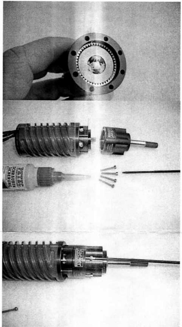
Turn the outputshaft. The gearbox must run without any jerk! Take care that you do not make a shortcut on the wires by holding the motor.
